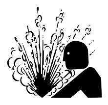
Explosive release of fluids from pressurized cooling system can cause serious burns.
